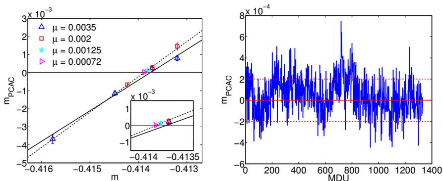
**Figure 2.** Left: PCAC mass versus  $\kappa$  in the tuning. Blue triangles are for the lattices  $N_s = 24$ , the red symbols for the lattices  $N_s = 32$ , the cyan star for a lattice of  $N_s = 32$  with a pion mass of  $m_\pi \sim 180$  MeV and the magenta point corresponds to the target ensemble with  $N_s = 64$ . Right: The history of the PCAC mass of our target lattice in units of molecular dynamics (MDU).
